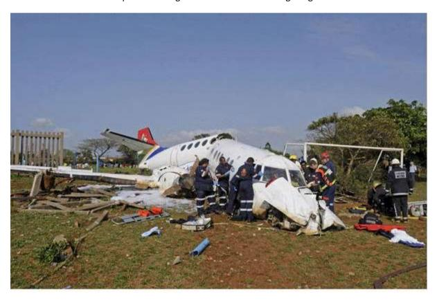
The aircraft crash landed following engine failure at take off and crashed into a concrete paling fence, see left hand side of the top photograph.
